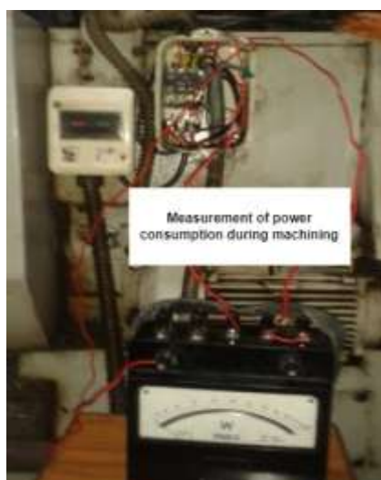
Fig. 2. Measurement of power consumption during machining
